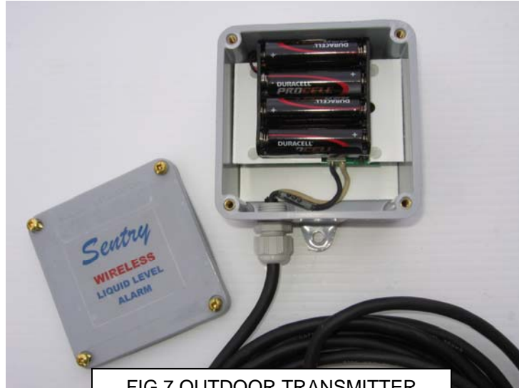
FIG 7 OUTDOOR TRANSMITTER BATTERIES INSTALLED
